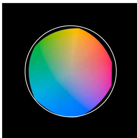
TM30 Colour distortion
